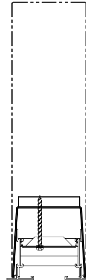
INSTALLATION WITH UP / UPL PLENUM, FIELD BUILT PLENUM, OR RETURN AIR APPLICATION
